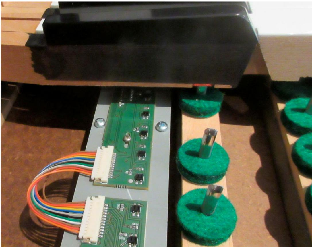
The edge of sensors rail must be at around 5mm from key pins board as photo above. Use 2 sharps near the ends of each circuit to ensure the best lateral centering, placing you at the vertical of keyboard to have the best global centering place under all black keys. Oblong holes are used for lateral precise adjustment.
