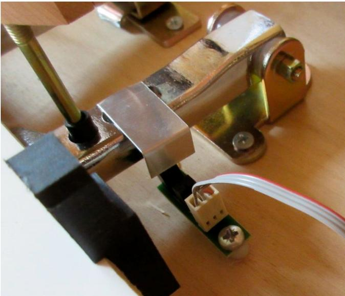
Screw the sensor with his white washer as shown on photo, use the aluminum part provided, cut and ply, glue with neoprene glue on top of the pedal, the vertical part has to go exactly in the center of optical fork. In the up position the sensor must be free opened. Connect the cable 1x6 table for two pedals, the pink wire indicating the damper pedal. The two slides on connector must be toward the optical fork sensor, if the connection is inverted, the pedal does not function.
